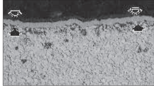
Surface of a WC – 11.5% Co cutting tool enriched with 1.9% Ta and 0.4% Nb (form complex carbides, the dark regions in the matrix) and coated with alumina (arrows) for enhanced tool life (Murakami's reagent, 1000X).
