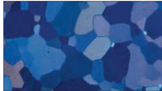
Grain structure of wrought, P/M beryllium (unetched, cross-polarized light, 100X).
