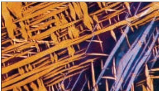
Mechanical twinning in deformed high-purity magnesium (99.8% Mg) (acetic-picral etch, crossed polarized light plus sensitive tint, 50X).
