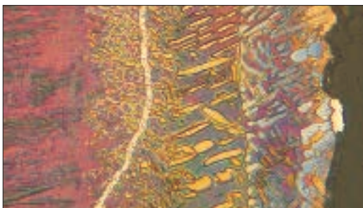
Alpha at the surface of heat treated (1038 °C, water quench) Ti - 3% Cr alloy after tint etching with Beraha's reagent (polarized light, 500X).
