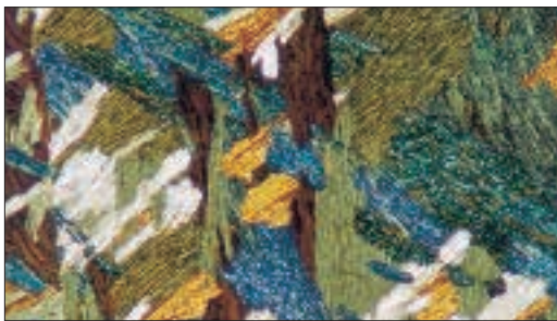
Basket-weave alpha-beta structure of as-cast Ti – 6% Al – 4% V revealed by heat tinting (polarized light, 100X).
